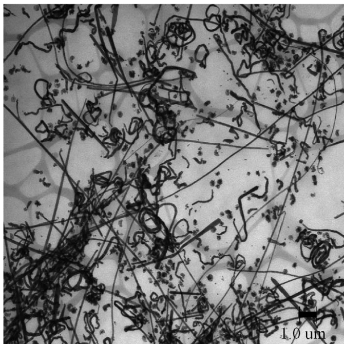
Fig. 3. A typical low magnification TEM image of silver nanowires obtained from tabular AgBr crystals after 5 min development.
